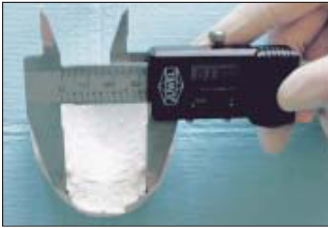
Fig 4 Width measurement on a dental cast using a fine-pointed digital calliper; approximation of all readings was made to the second decimal place.
