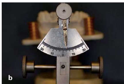
Fig 4 (a) Torque measurement with the Model-Checker. (b) Tip measurement with the Model-Checker.
