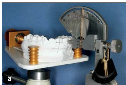
Fig 4 (a) Torque measurement with the Model-Checker. (b) Tip measurement with the Model-Checker.
