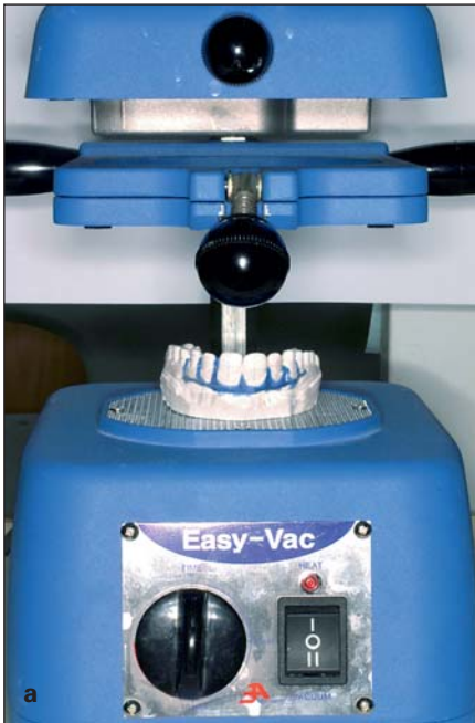
Fig 10 Vacuum former is used to make (a) the 0.020-inch-thick Clear Aligner and (b) the 0.030-inch-thick Clear Aligner.
